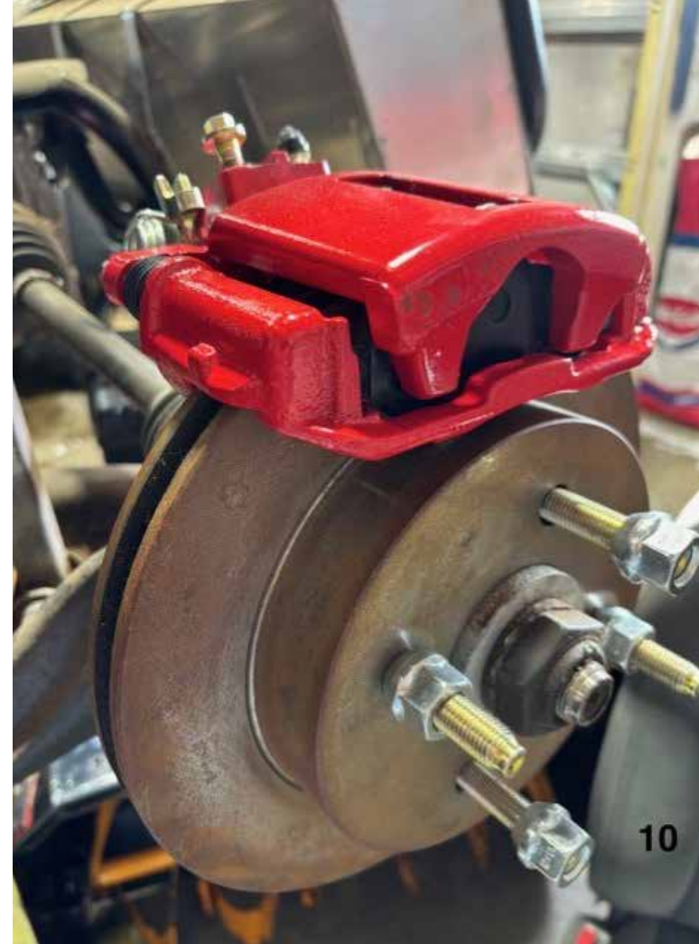
Pictures 10 & 11 show the finished product with the mount and caliper painted and ready to be piped. I got all the brake fittings I needed to connect all the different components together from Amazon: great quality parts and way cheaper than the online brake specialists. Summit Racing in the USA had pre-made braided stainless lines which will fit all four corners. That'll be the next update.
