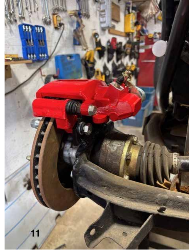
Pictures 10 & 11 show the finished product with the mount and caliper painted and ready to be piped. I got all the brake fittings I needed to connect all the different components together from Amazon: great quality parts and way cheaper than the online brake specialists. Summit Racing in the USA had pre-made braided stainless lines which will fit all four corners. That'll be the next update.
